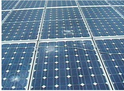
Figure 2: Baseballs cause starburst breakage patterns in the module glass and can damage underlying cells.
